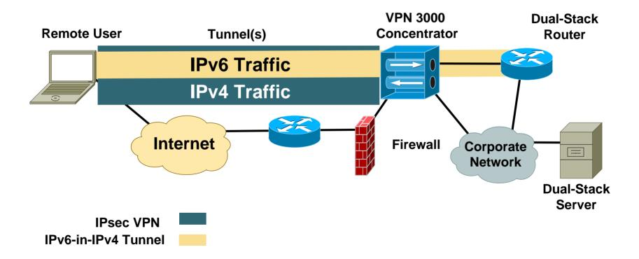
Note: The VPN concentrator could be replaced with a VPN-enabled Cisco IOS Router or PIX™
